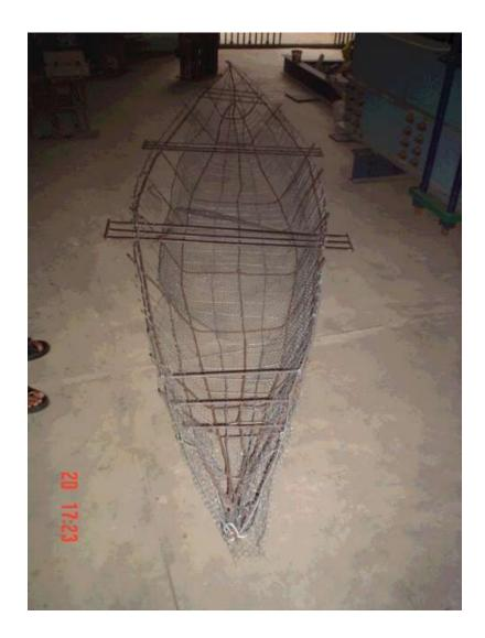
Figure 7. Skeleton of the first prototype ferro-cement boat under construction in KIIT workshop.
