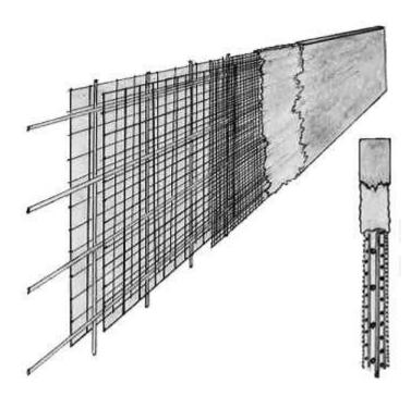
Figure 1. Schematic diagram of typical ferro-cement sheet.
