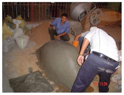
Figure 6. Model ferro-cement boat being finished.
